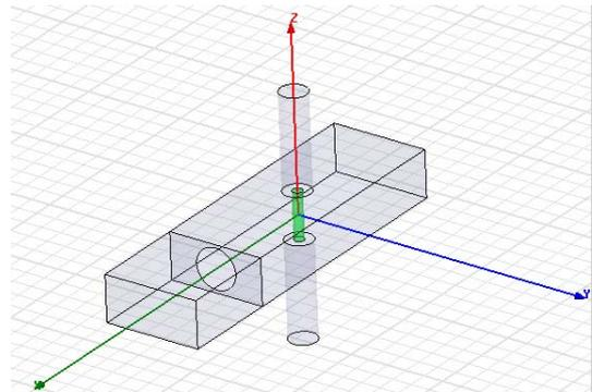
Figure 1. Geometry of the TE<sub>103</sub> resonant cavity
