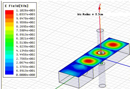
Figure 3. Electric field distribution for the optimum iris size
