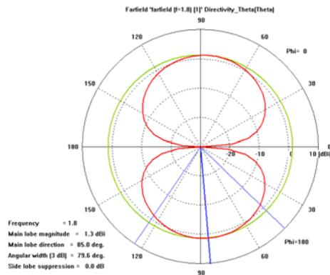
**Figure 7.**  $E_\phi$  and  $E_\theta$  radiation patterns of the PIFA mounted antenna
