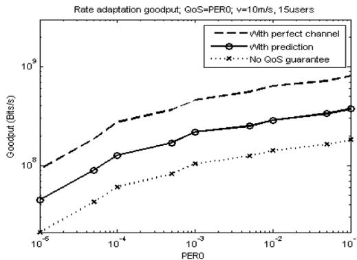
Figure 7 Goodput comparison in multi-rate transmissions
