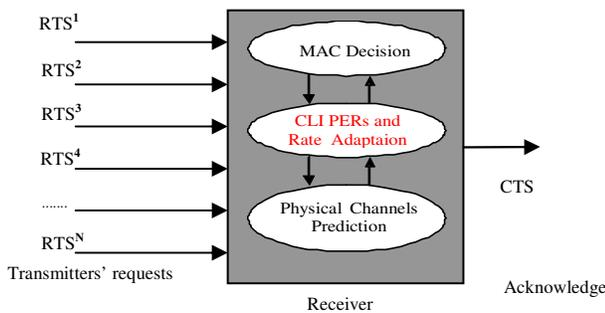
Figure 2 The handshaking mechanism for QoS
