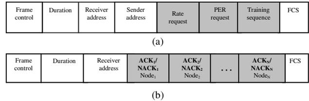
Figure 3 a) RTS control packet b) CTS control packet
