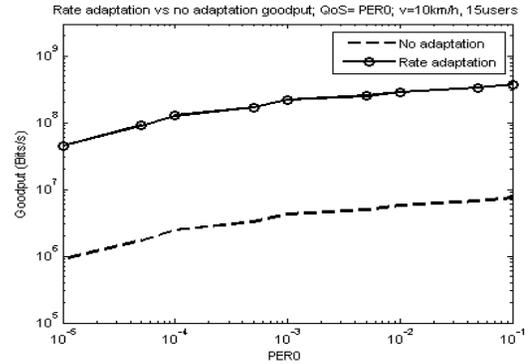
Figure 5 Goodput comparison of multi-rate rate vs single-rate in clairvoyant transmissions
